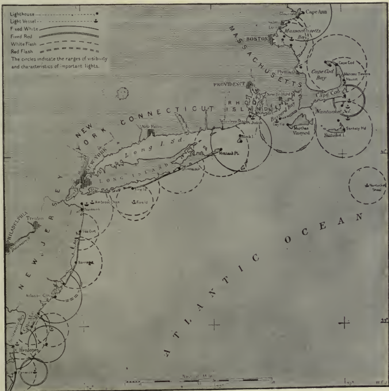
General lighting of Atlantic coast at entrances to Boston, New York, and Philadelphia.
